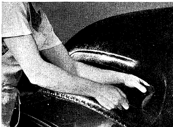
Fig. R.10. Cutting surplus material from the back window aperture prior to tacking.
